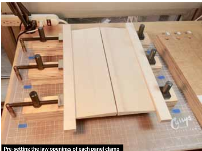
Pre-setting the jaw openings of each panel clamp
