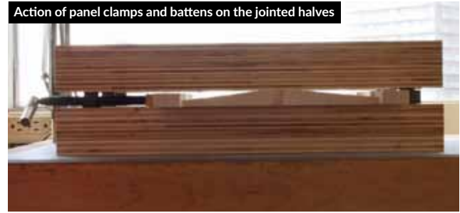
Action of panel clamps and battens on the jointed halves
