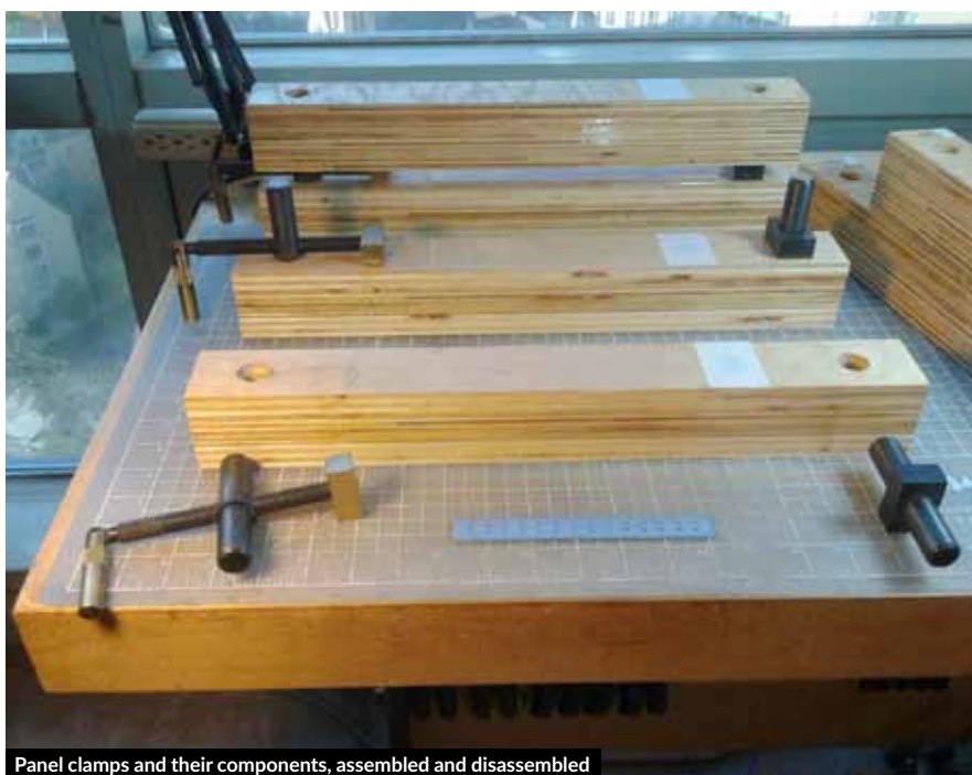
Panel clamps and their components, assembled and disassembled
