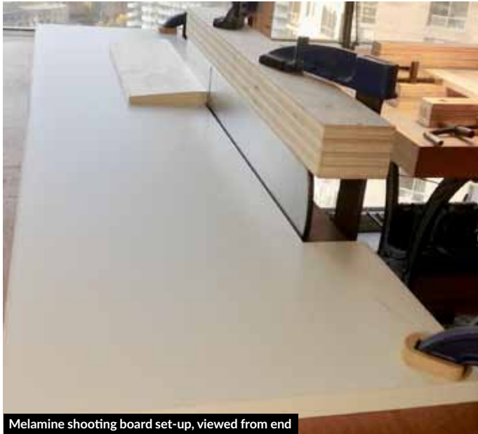
Melamine shooting board set-up, viewed from end
